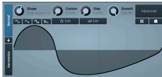
Figure 7: Skewed sinusoidal LFO shape used in the Melda Phaser and Flanger irregular LFO effect modeling experiments.
